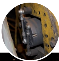
Leine & Linde heavy-duty encoder is installed on one of the mining locomotives.
